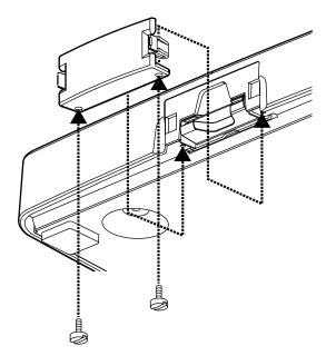
When removing the card cover, remove only the specified screws.
